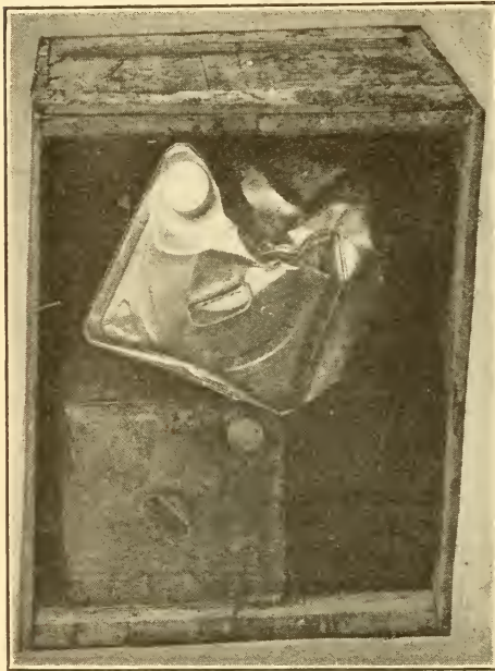
A honey can after being shipped loose in a box. Most of the honey had leaked out.
